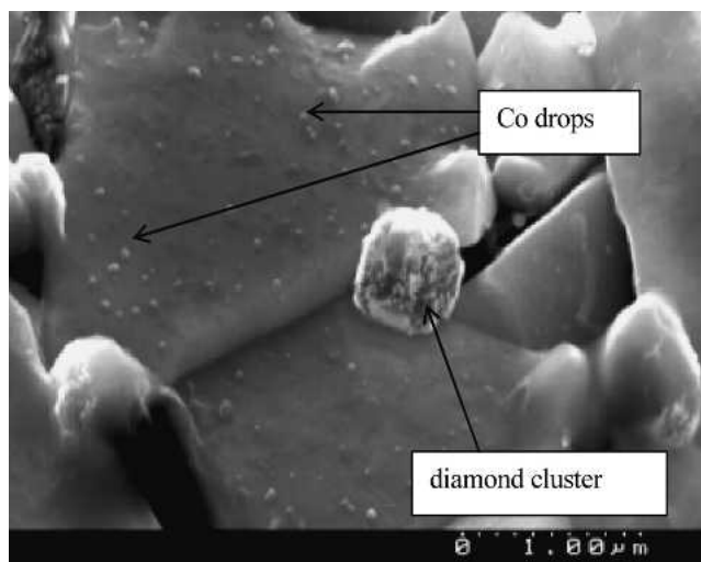
Fig. 5 SEM micrograph showing the surface of the coarse-grain substrate after 15 min of BEG
